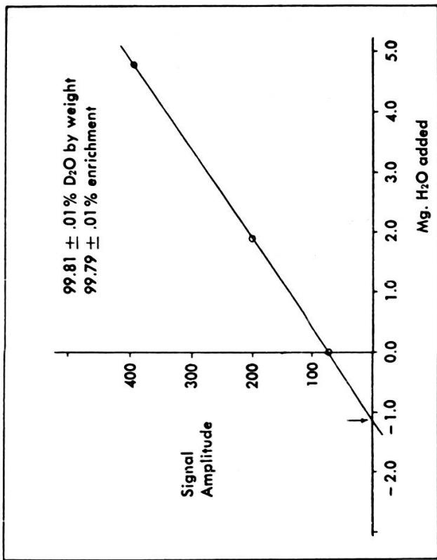
H<sub>2</sub>O Remaining in High Purity D<sub>2</sub>O by the Method of Adding Known Amounts of H<sub>2</sub>O and Extrapolating to Zero Signal Amplitude.
