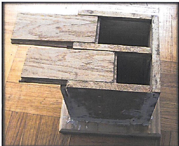
Fig. 8. Top of the tank, hatches and partition.
