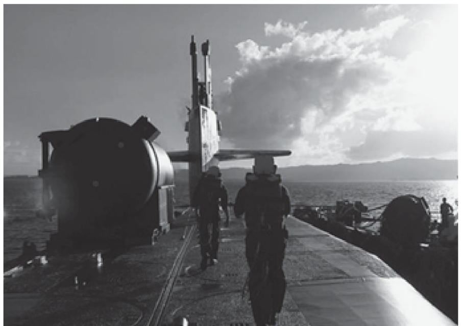
Four former strategic ballistic missile submarines of the Ohio-class were recently converted to cruise-missile and Special Operation Forces carriers. They each have 154 Tomahawk cruise missiles aboard and thus offer a unique strike power to the operational U.S. commanders worldwide. Photo: US DoD
