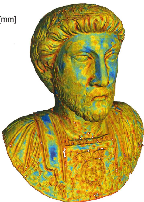
Fig. 6 Thickness map of the golden bust of Marc Aurel determined by neutron tomography investigations at the NEUTRA neutron imaging beam line at SINQ (PSI). Cf. De Pury-Gysel/Lehmann/Giumlia-Mair 2016.
