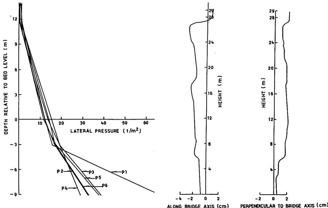
FIG. 2 (a) LATERAL PRESSURE VALUES OBTAINED FROM PRESSURE CELLS ( $t/m^2$ )
