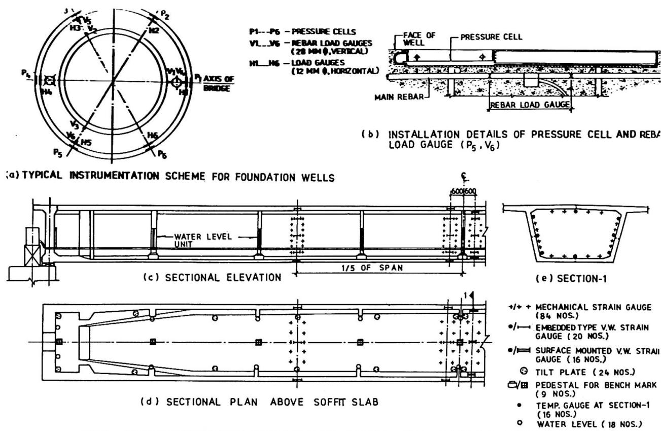
FIG. 1 INSTRUMENTATION SCHEMES FOR GANGA AND MANDOVI BRIDGES
