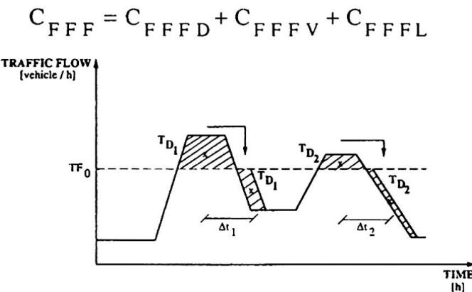
Fig. 1 Simplification proposed for the traffic flow curve versus time of the day
