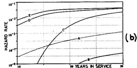
a) Sequence : 680 B in fatigue followed by 611 B in fatigue b) Sequence : 680 B in fatigue followed by 620 under an extreme wave. Notation : A-no inspection (design stage) B-no crack is found C-14mm crack is found D-Through thickness crack is found E-Section is found to have failed.
