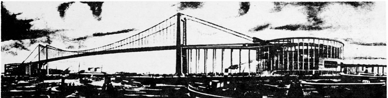
Fig.3 A bridge with spiralttype access structures as proposed for the Maastunnel in Rotterdam.
