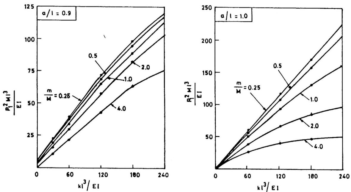
FIG. 3 VARIATION OF FIRST BENDING FREQUENCY
