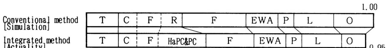
T:Temporary-work, C:Concrete-work, F:Form-work, R:Re-Bar Placing-work, F:Finish-work, EWA:Utility, P:Piling-work, L:Landscaping, O:Others
