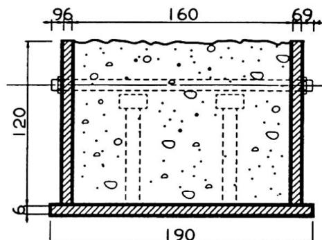
Fig. 1. Loading arrangement and the cross-section of the tested arches.
