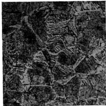
Thermally altered structure, ferrite and sorbite, transition zone.
