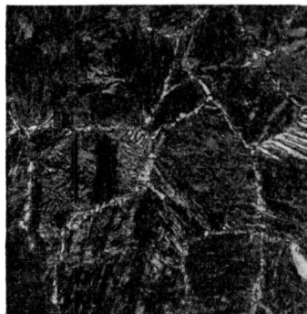
Not pre-heated, formation of Martensite.
