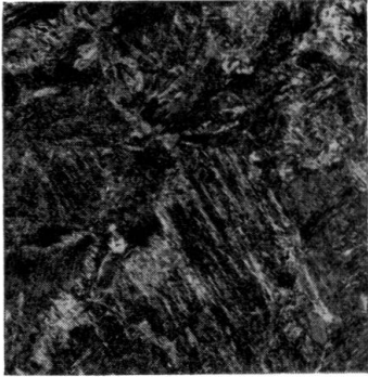
Temperature: -10^{\circ} C. Martensite with traces of troostite due to quenching effect.
