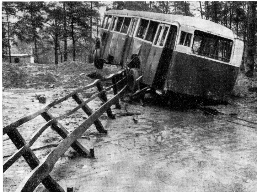
FIG. 7. Heavier parapet of the Royal Board of Roads and Waterways after the bus has run against at an angle of 45°. The bus has slid above the parapet and stopped on the right side, after one front wheel had touched the ground in front of the parapet for a moment.
