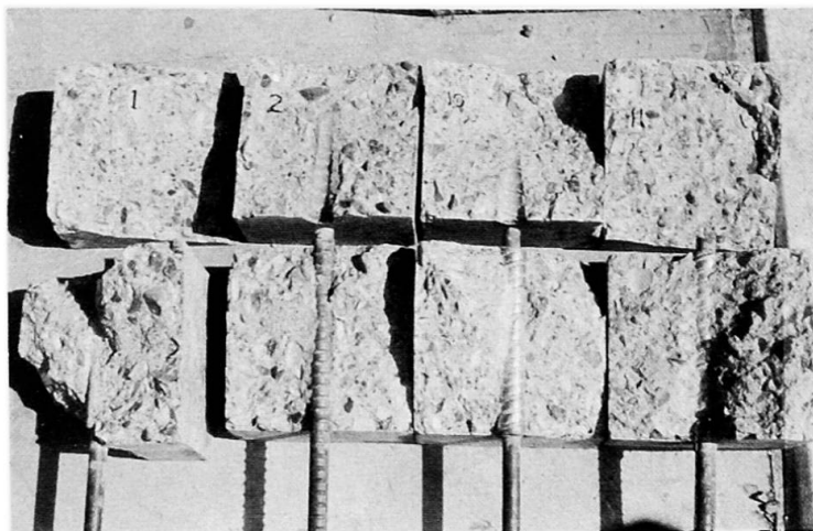
Phot.1 Inside of specimens after pull-out bond test
