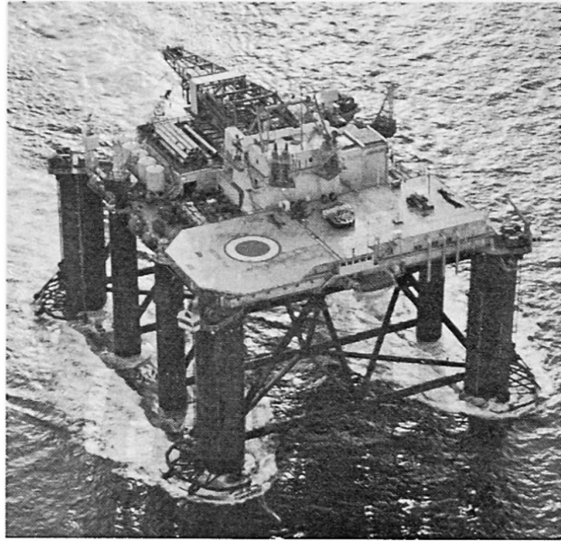
Fig. 5. Twin-hull supported Semi-submersible
