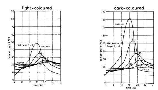
Fig. 3 Thermal stress of outer wall with light and dark colour, according to [5].
