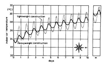
Thermal cyclic behaviour of a west-orientated room of light and heavy construction, according to [3]. Basic data 40 % window surface clear insulation glazing with outer blind change of air 0,5 h<sup>-1</sup>
