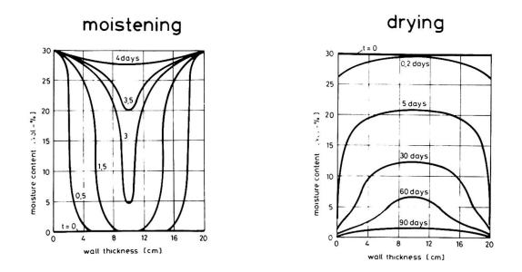
Distribution of moisture concentrations on a wall of cellular concrete Fig. 5 at different instants, according to [6]. On the left: Moistening on both sides (sucking, rain), On the right: Drying on both sides.
