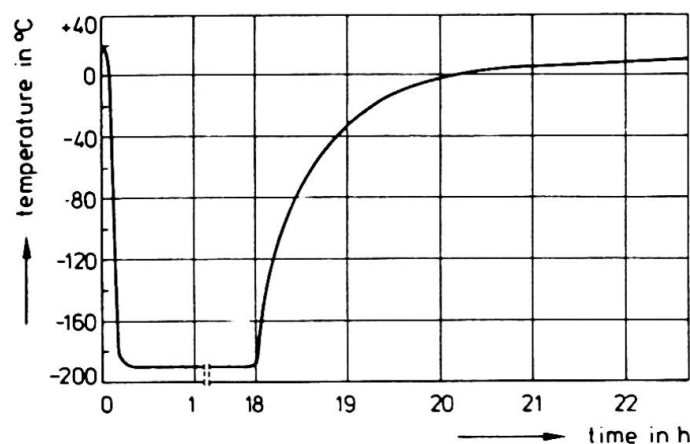
Fig.3 Temperature exposure of "low-temperature-specimens"
