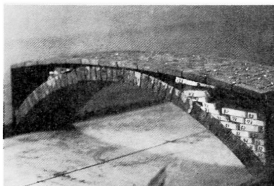
Photo 4 Collapse of arch spandrel of downstream side.
