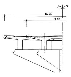
Final Solution (Road axis constant): thickening of existing slab and introduction of additional ordinary steel reinforcement over the longitudinal beams.
