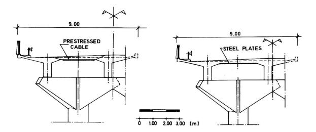
1st Solution (Road axis changes): DYWIDAG 20F strand cables spaced 0.50 m in the longitudinal direction anchored at the top of the slab. The anchorages are to be sealed with epoxy mortar. 2nd Solution (Road axis changes): steel plates with 2800x250x4 spaced 1.00 m in the longitudinal direction glued and riveted to the concrete.
