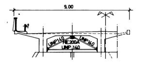
3rd Solution (Road axis changes): metallic frames spaced 2.00 m in the longitudinal direction on top of which rests a HE200A beam. The frames are connected to the longitudinal beams through plates riveted to the concrete.
