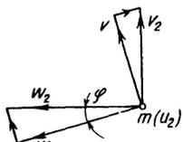
$$\left. \begin{aligned} U &= U_2 \\ V &= V_2 \cdot \cos \varphi + W_2 \cdot \sin \varphi \\ W &= W_2 \cdot \cos \varphi - V_2 \cdot \sin \varphi. \end{aligned} \right\} \quad (7)$$
