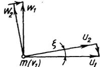
$$\left. \begin{aligned} U_2 &= U_1 \cdot \cos \zeta + W_1 \cdot \sin \zeta \\ V_2 &= V_1 \\ W_2 &= W_1 \cdot \cos \zeta - U_1 \cdot \sin \zeta. \end{aligned} \right\} \quad (6)$$
