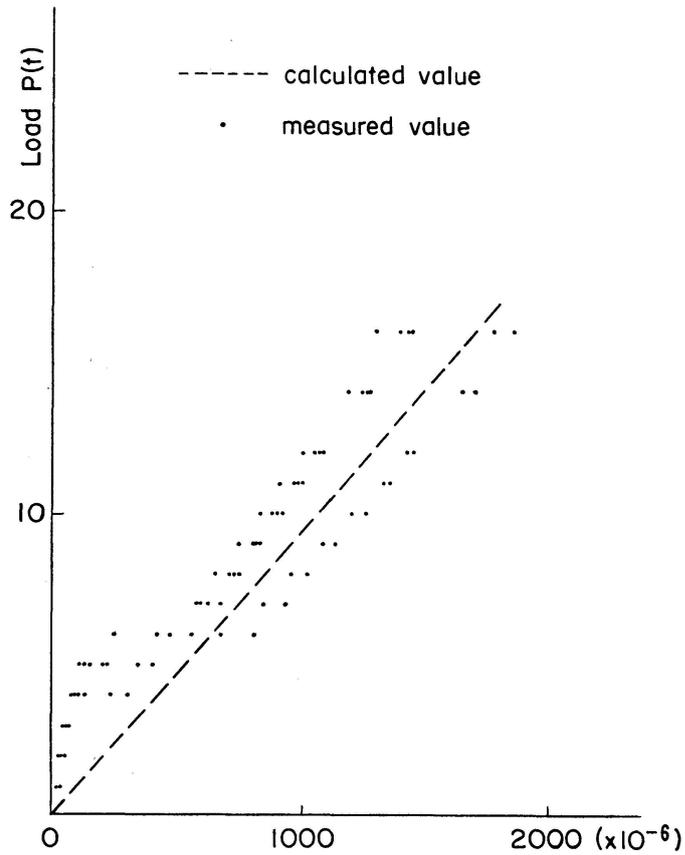
Fig. 4. Strain of reinforcement in beam A 2.
