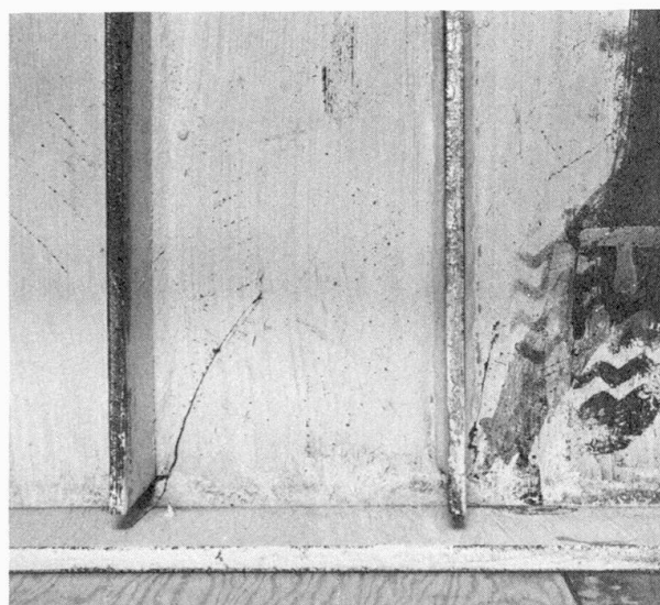
Fig. 7. Typical Failure at Web Stiffeners.
