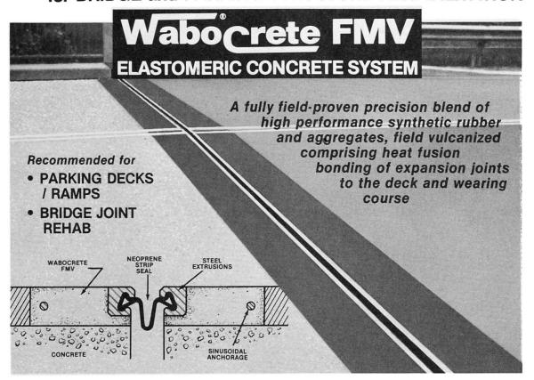
WABOCRETE FMV is ideal for lane-at-atime rehabilitation work. Its rapid installation and heat fusion vulcanizing require about 2 hours. It serves as an energy absorbing, spall & crackfree, impervious expansion joint end dam in one piece from curb to curb.
