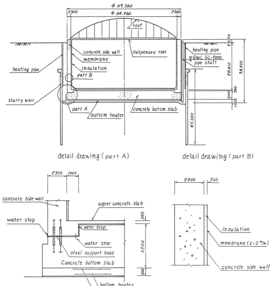
Fig. 1 Cross section with details
