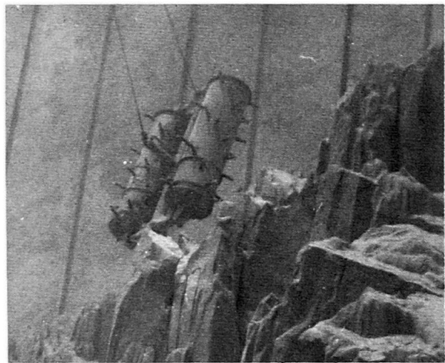
Fig. 1 Potash hanging up on silo wall (It will not flow prior to installation of reclaim system)
