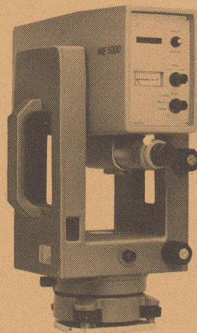
The remarkable accuracy of this instrument –  $\pm (0.2 \text{ mm} + 0.2 \text{ mm}/\text{km})$  – is based on the use of a helium-neon-laser beam and one single crystal for modulation and demodulation. At distances exceeding 200 m, the Mekometer, an 11 kg featherweight, easily outperforms one-second theodolites in point surveys.
