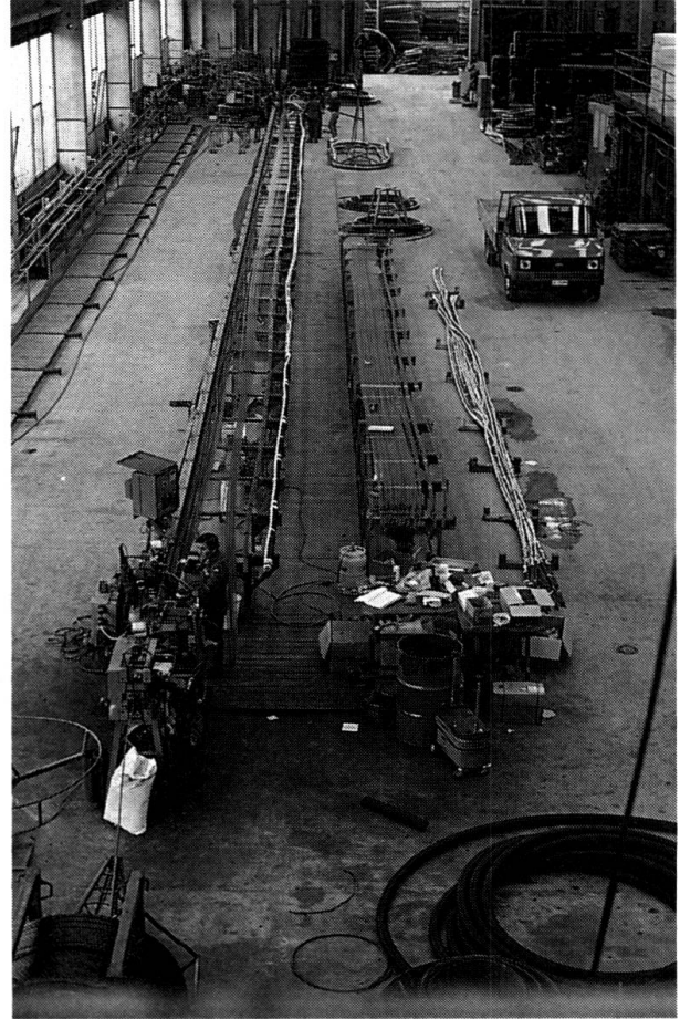
Fig. 2 Fabrication of the anchors in the VSL workshop
