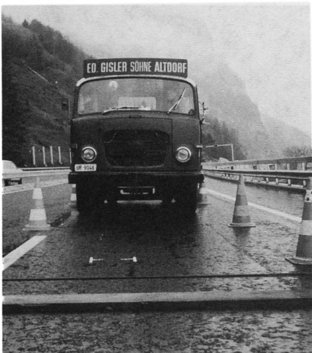
Fig. 3 A two-axle test vehicle before passing over a contact threshold (speed measurement) and over a plank.
