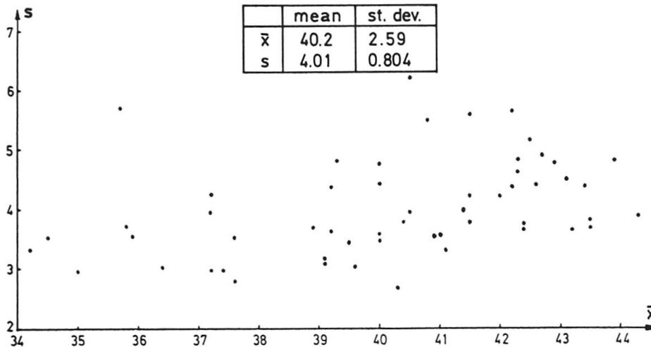
Fig.4 Characteristics of the production of Belgian ready-mixed concrete plants ( $f_{ck, cub} = 27.5 \text{ N/mm}^2$ )
