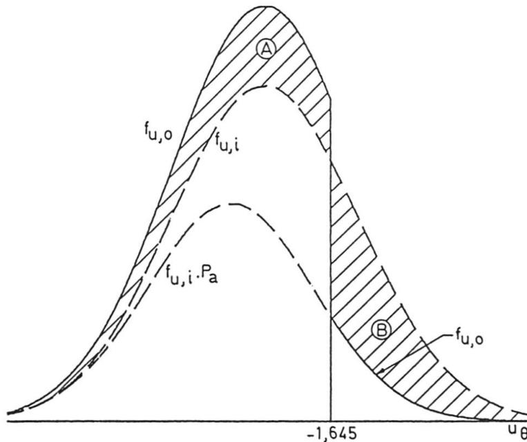
Fig.14 Filtered process curve taking into account rejected lots
