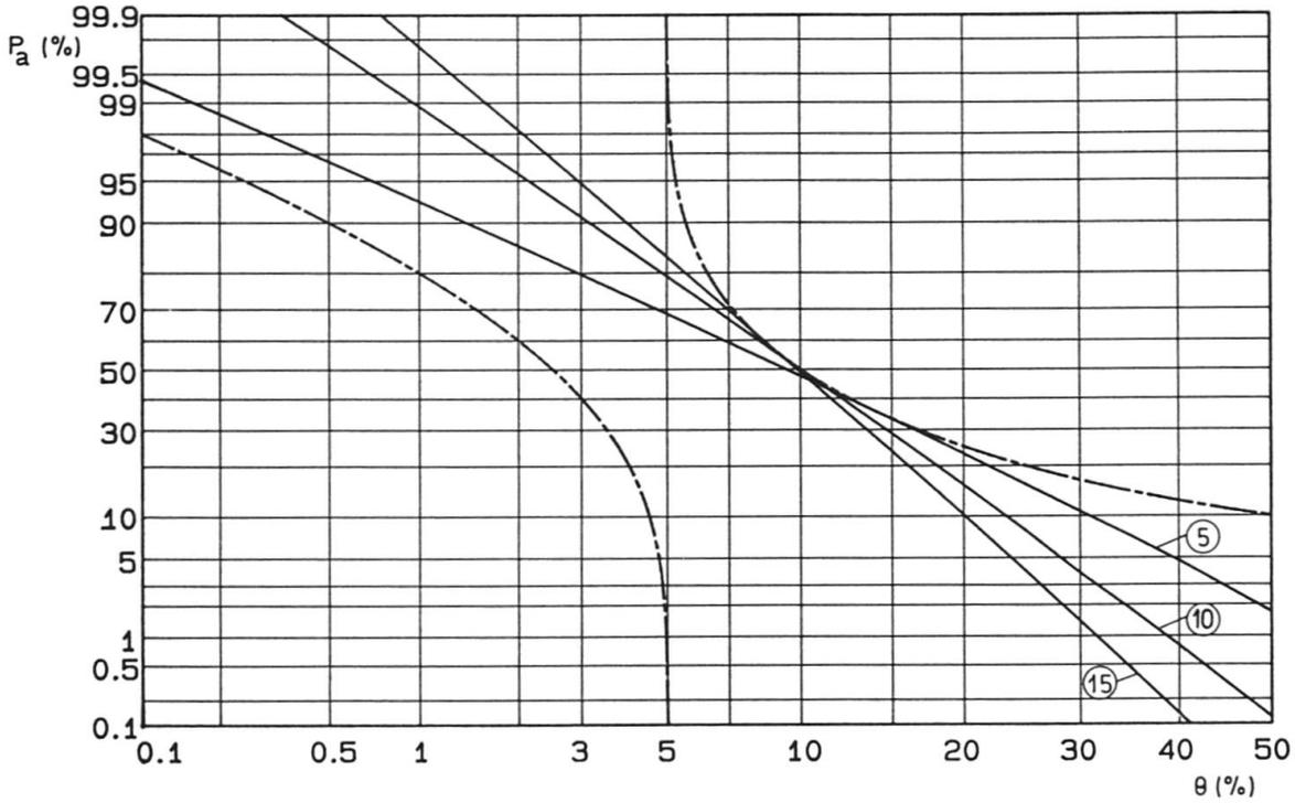
**Fig.12** Criterion  $\bar{x}_n \geq f_{ck} + \lambda s_n$  ( $n=5, 10, 15$ ). OC-lines tangent to the unsafe region
