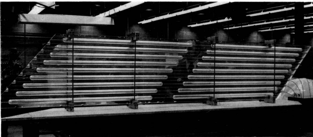
Figure 21 - Two Span Plexiglass Model of a Post-Tensioned Voided Skew Bridge Slab (1/24)
