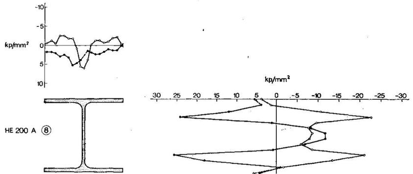
Fig. 6 Residual stresses in an HE 200 A shape rotorized twice
