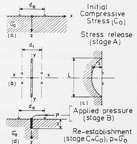
consists in a local elimination of stresses, followed by a controlled stress compensation (fig. 1). In practice, the displacement reference field is first determined; a slot is then cut in a plane normal to the desired direction of stress determination; finally, a very thin flat jack is introduced into the slot and used to restore the initial displacement field. The amount of cancelling pressure is an indication of the compressive stress in the direction normal to the slot.
