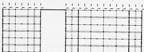
Vertical unbonded horizontal bonded reinforcement
