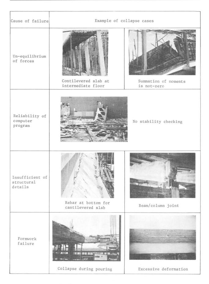
Fig. 2 Collapse case of super-structures
