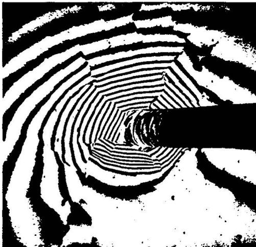
**Fig. 7.** Localized splitting cracks at end-face, experimentally [3].
