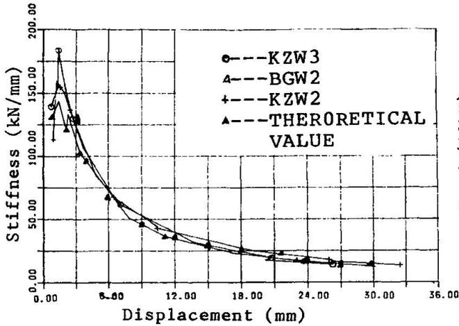
Fig.6 Stiffness Degradation
