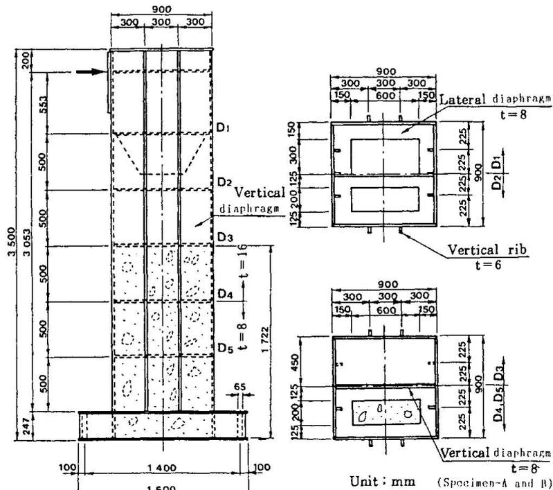
Fig. 2 Configuration of specimens
