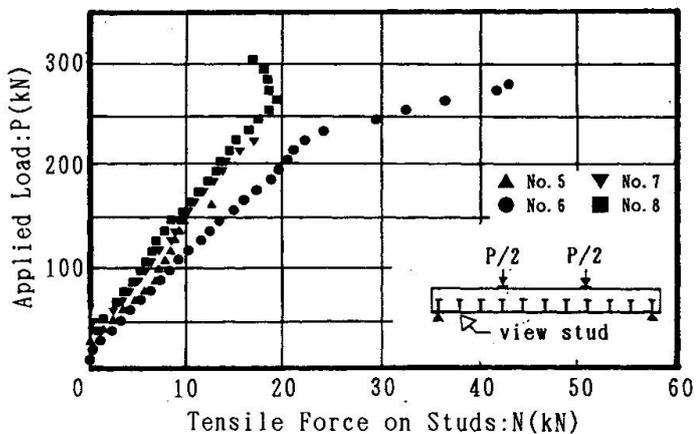
Fig.8 Tensile Forces at the Body of Studs
