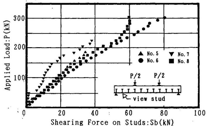
Fig.7 Shearing Forces at the Base of Studs
