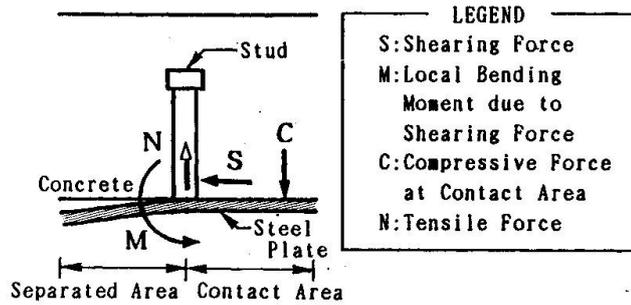
Fig.6 Mechanism of the Tensile Force in Elastic Region
