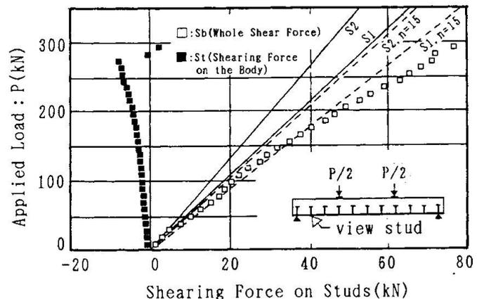
Fig.9 Shearing Forces at the Base
