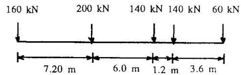
Figure 1. Details of Bridge Model and Loading.
