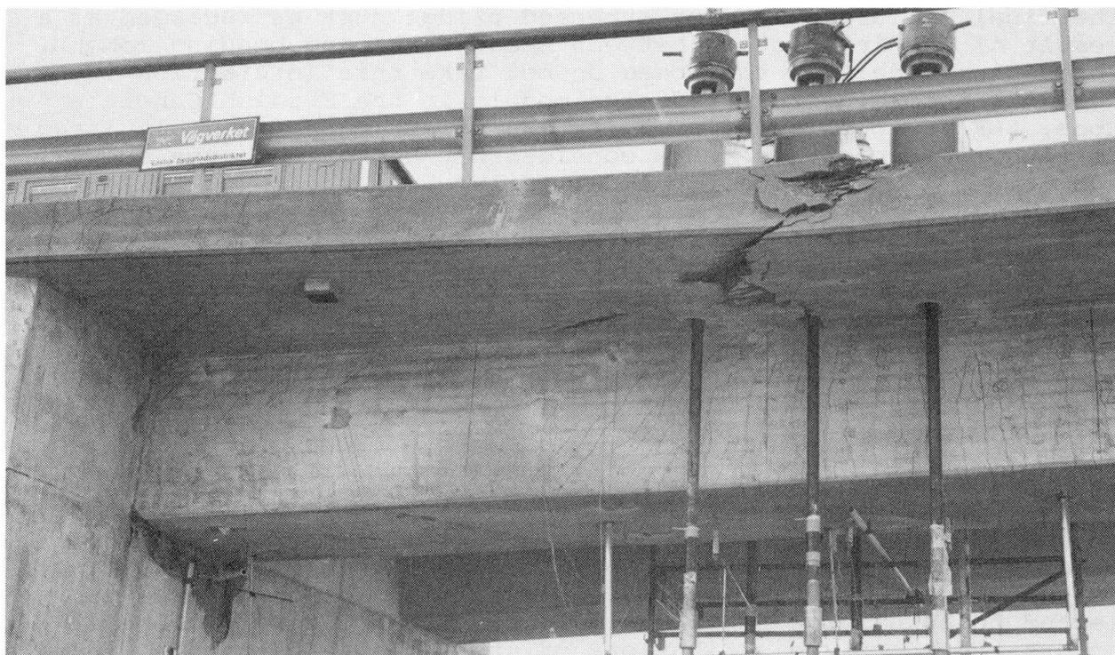
**Fig. 7** Failure in the prestressed bridge. Cracking, support failure and concrete compression failure at the top of the loading section can be seen.
