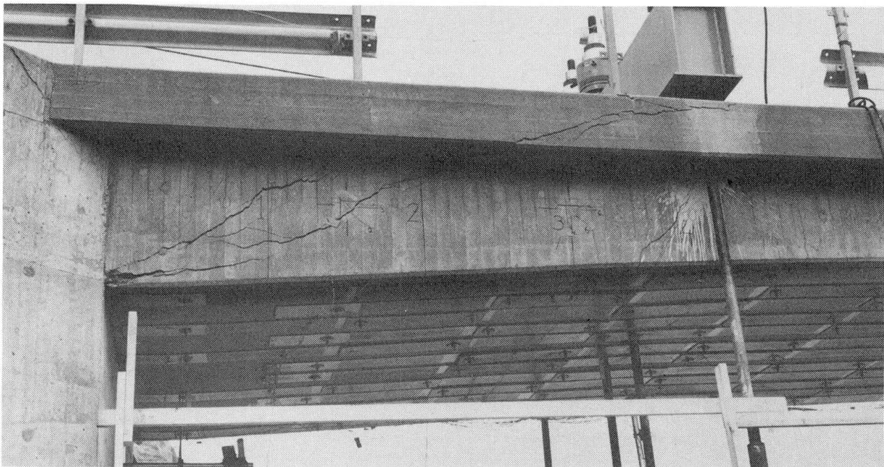
Fig. 6 Shear failure in the non-prestressed bridge
