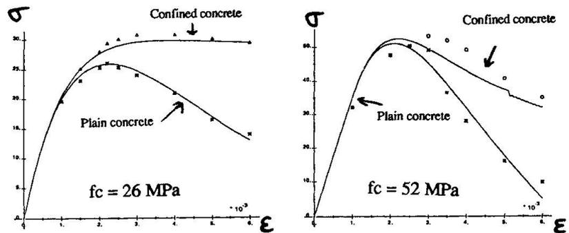
Fig.7 Stress-strain curves — numeric
