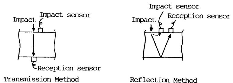
Fig. 4 Standard Measuring Method [4]
