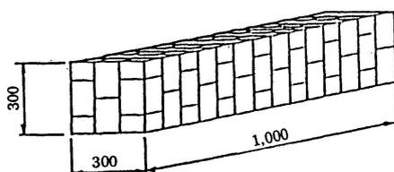
Fig. 5 Dimensions of Brick Specimen
