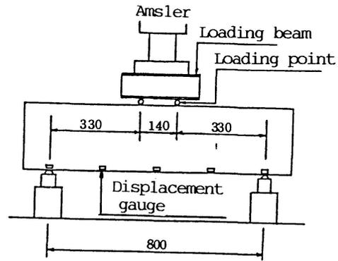
Fig. 7 Loading Device and Loading Points (unit: mm)
