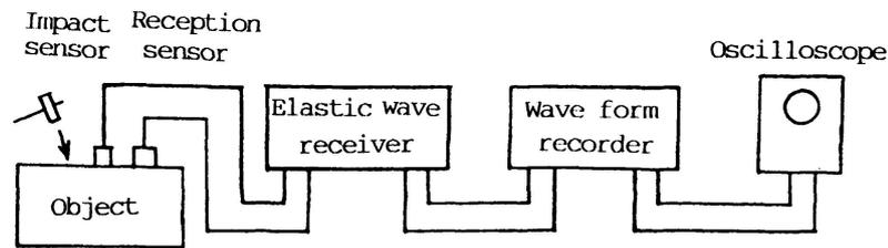
Fig. 3 Standard Configuration of Elastic Wave Measurement System [4]
