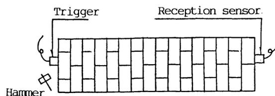
In measuring reflected waves, the trigger and the reception sensor are positioned at the corresponding points on the opposite faces.
