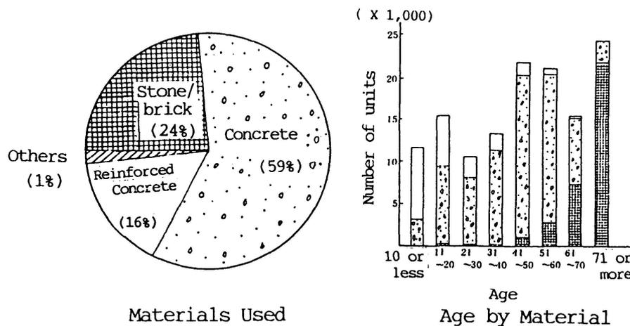
Fig. 1 State of Substructure (132,000 units)
