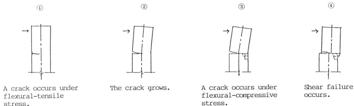
Fig.10 Failure Process [5]
