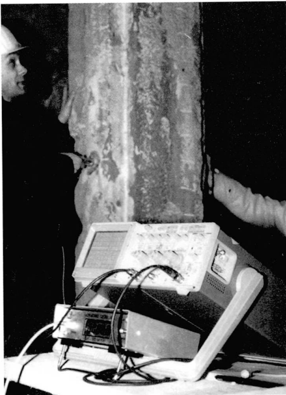
Fig. 7: Investigation of a sandstone pillar with the ultrasonic method
