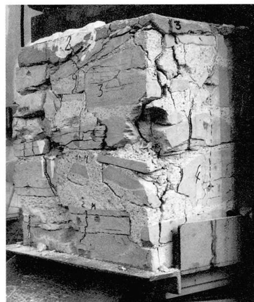
Photo 7 - Collapse of specimen No. 3.
