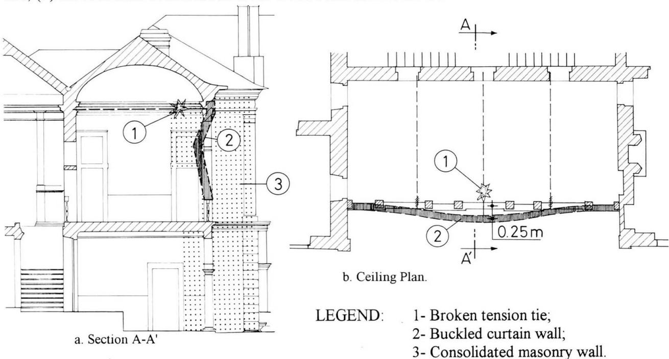
Fig. 6 - North Loggia Facade Collapse Mode.
