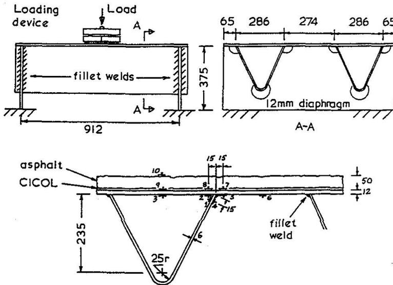
Fig. 5 Full scale test by Smith et al. [9]
