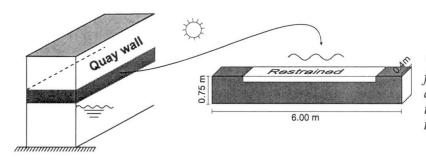
"Presentation of practice oriented full scale experimental research and the restrained temperature induced deformations at the top of the beam"
