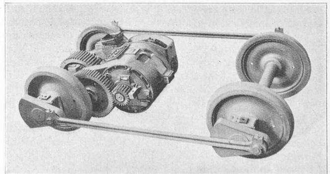
Fig. 3. — Truck des locomotives Ee 2/2.
