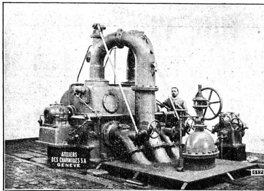
**TURBINE PELTON A 2 ROUES, 4 JETS, 650 CV.**
