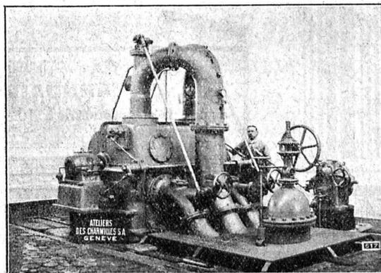
**TURBINE PELTON A 2 ROUES, 4 JETS, 650 CV.**
